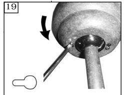
Lift Canopy to ceiling aligning the key hole slots with the screws on the bottom of the Mounting bracket. Rotate the canopy Counter Clockwise to lock in place. Tighten the screws to secure the Canopy. See inset for Keyhole shape
